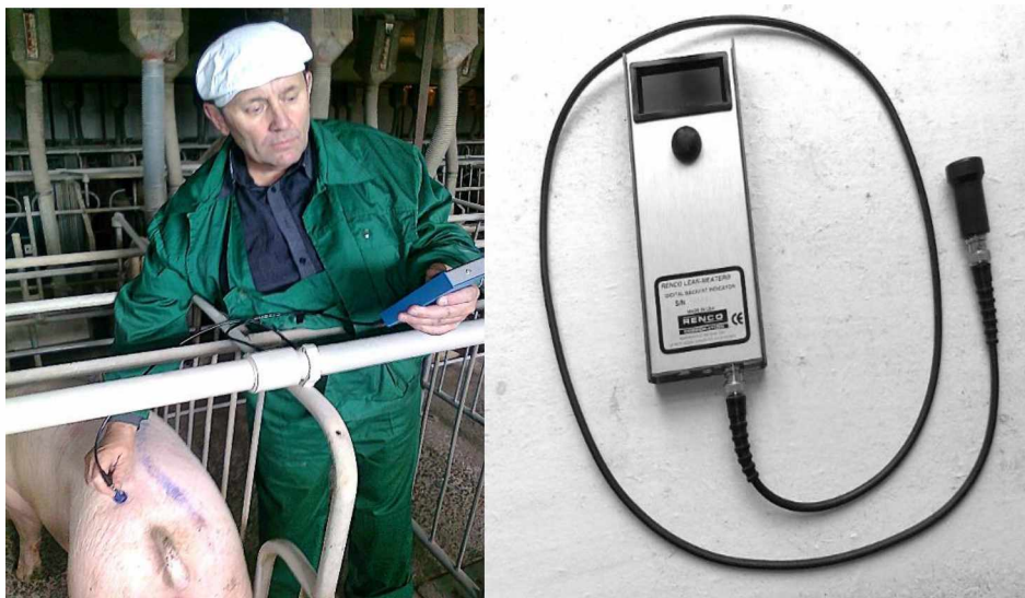
Fig. 1. Measurement of lard thickness with the RENKO CE device (RENKO LEAN MEATER DIGITAL BACKFAT IDIC, S/N 46080)
